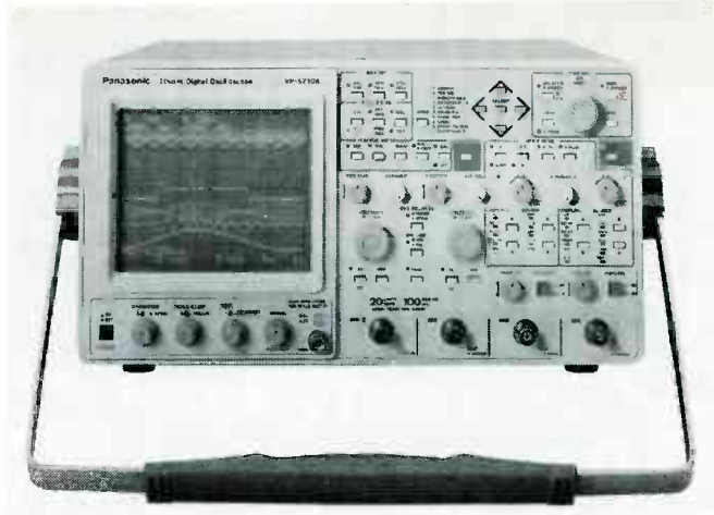
PANASONIC'S VP-5710A is a menu-driven, 4-channel DSO with a large 64K memory. A unique display position lets you view a large part of the signal on the top of the screen, with a small portion of the waveform below it.
